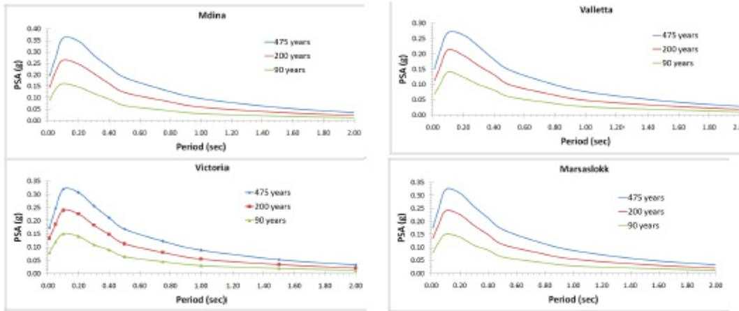
Figure 4: mean UHRSA for 90, 250, and 475 years return periods for the whole logic tree computed at four different locations on the Maltese islands
