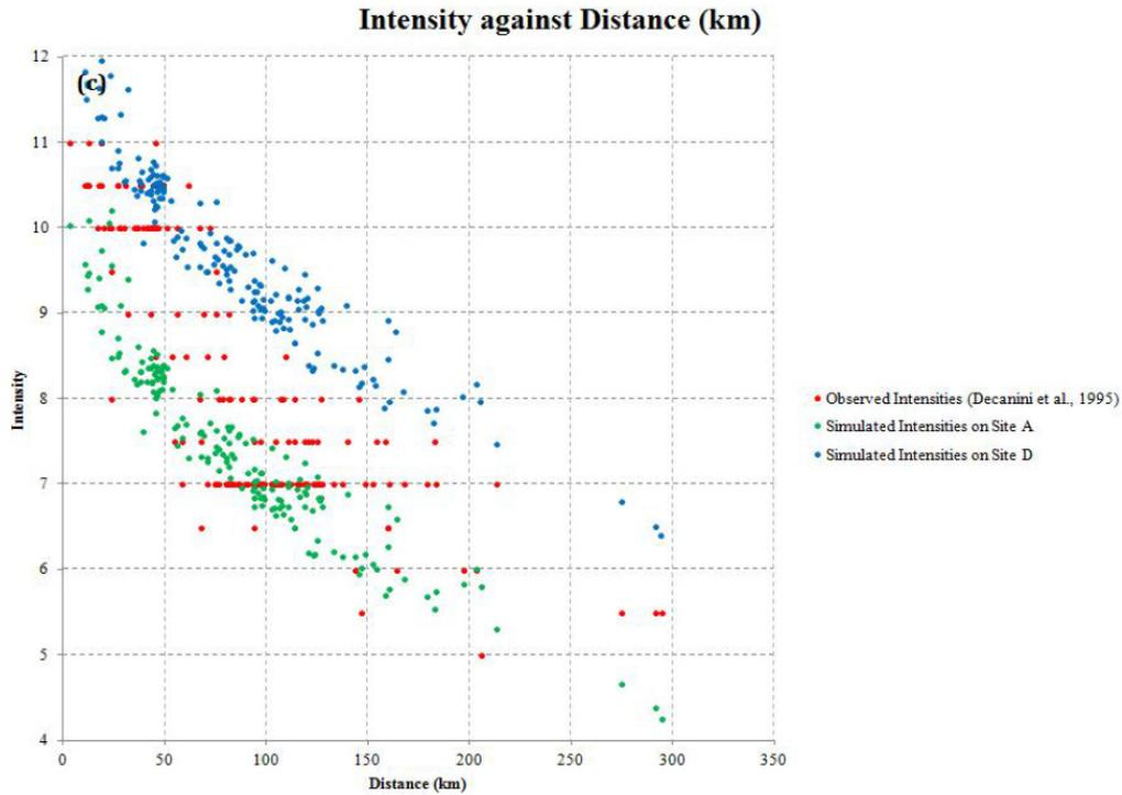
Figure 9: Intensity values at Sicilian localities (red dots) listed in the DBMI11 database for the 11/01/1693 earthquake compared with intensity values converted from the simulated PGA curves.
