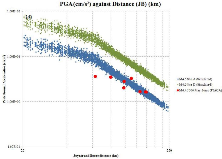
Figure 8: Observed PGA values from accelerometric data from a M4.4 event in the Ionian Sea. Recorded at stations in Sicily, and compared with theoretically simulated ground motion.
