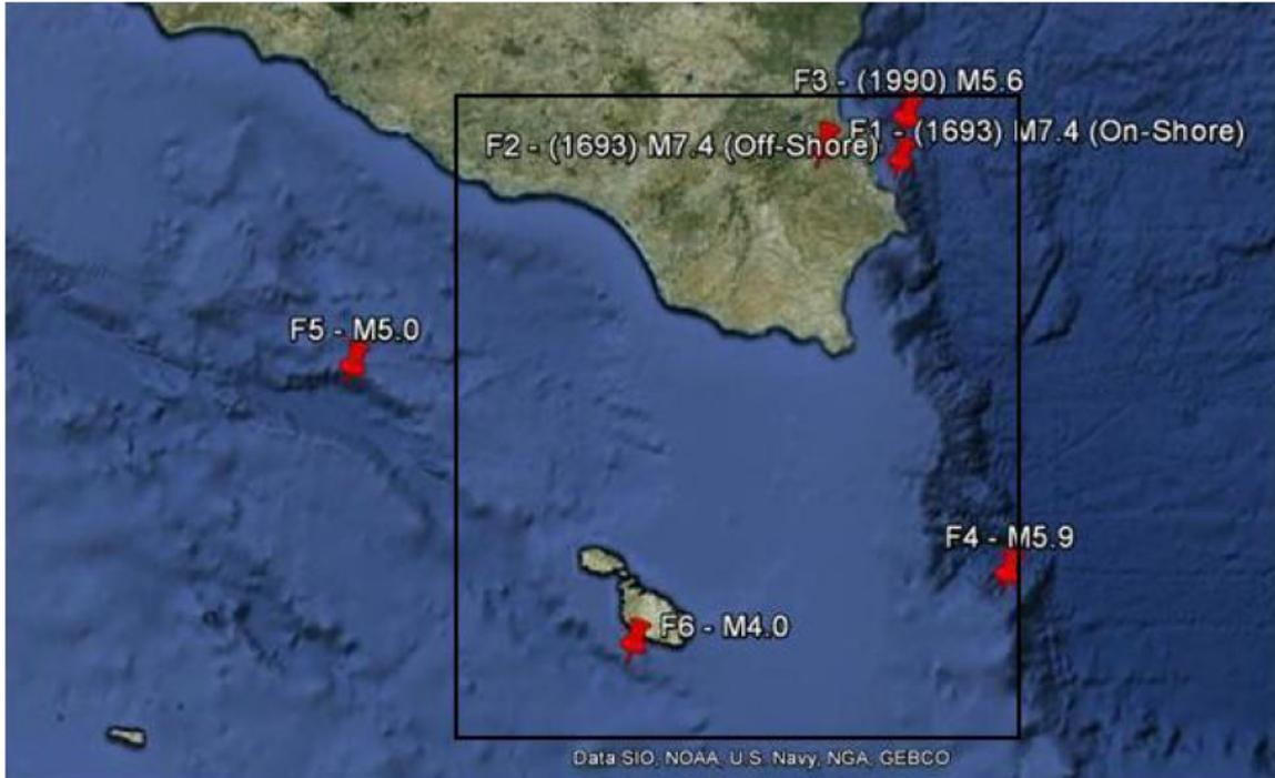
Figure 6: The hypothetical fault sources used in the regional earthquake simulation exercise for obtaining attenuation relations. The square shows the edges of the grid of sites at which the simulations were computed.
