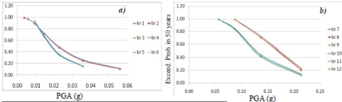
Figure 2. Hazard curves (at the bedrock) for Malta using the logic tree approach
