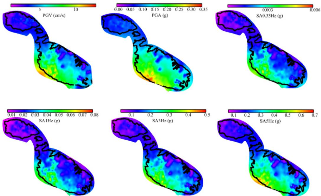
Figure 3: Ground motion scenarios for earthquake of Mw = 5:0 located about 20k south of Malta.
