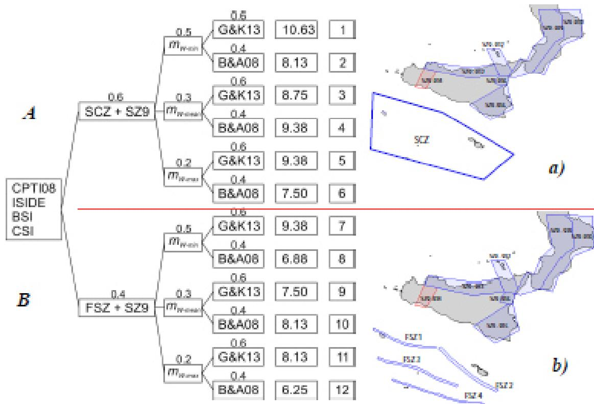
Figure 1. Logic Tree approach used and seismogenic sources used in the present study. We employed two different attenuation relationships: G&K13(Grazier and Kalkan, 2013) and B&A08 (Boore and Atkinson 2008)
