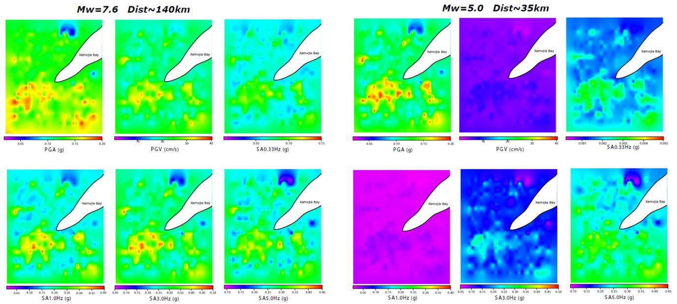
Figure5: The maps show the ground motions for (left group) a M7.6 earthquake scenario event at about 140km from the study area and (right group) a M5.0 earthquake at a distance of 35km from the study area. The figures show PGA, PGV and Spectral Acceleration at different frequencies.
