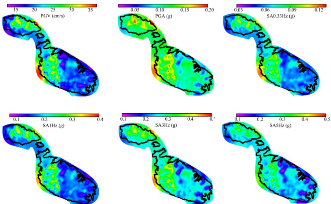
Figure 2: Ground motion scenarios for earthquake of  $M_w=7.6$  located on the Hyblean-Maltese escarpment.
