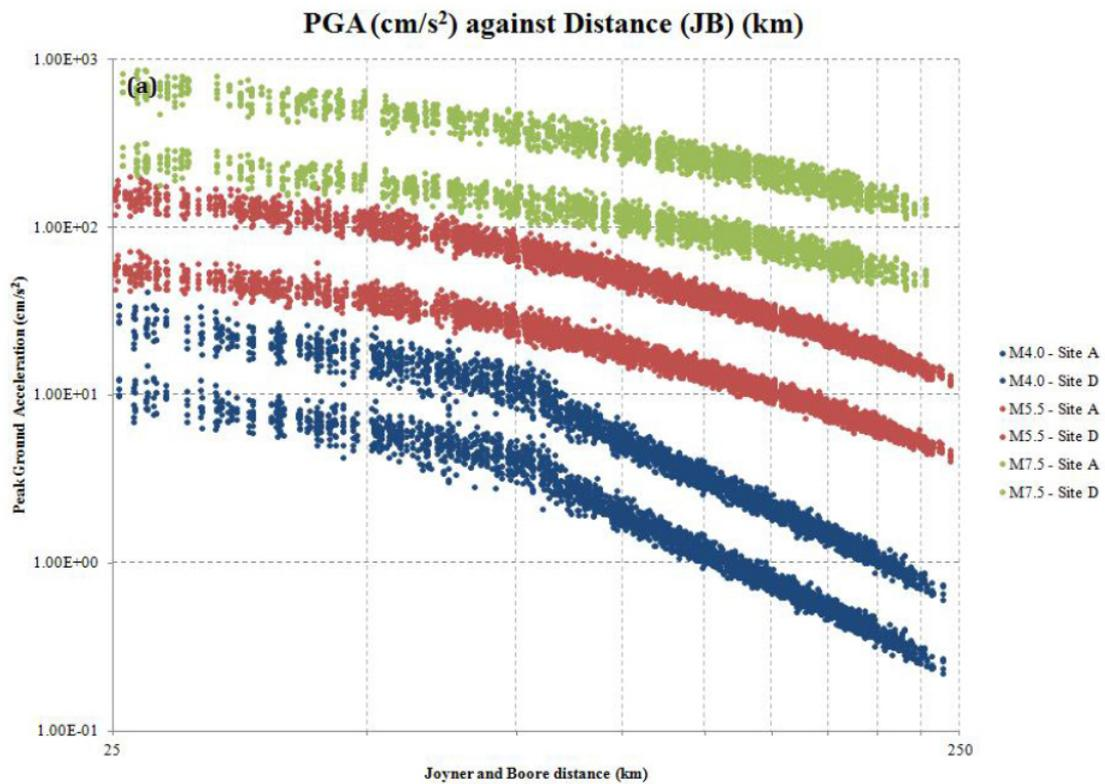
Figure 7: Theoretically computed PGA values for earthquakes of magnitudes 4.0, 5.5 and 7.5, at site classes A and D. Each point of the graphs represents a ground motion simulation for a different set of parameters (depth, magnitude, distance, site class, etc)
