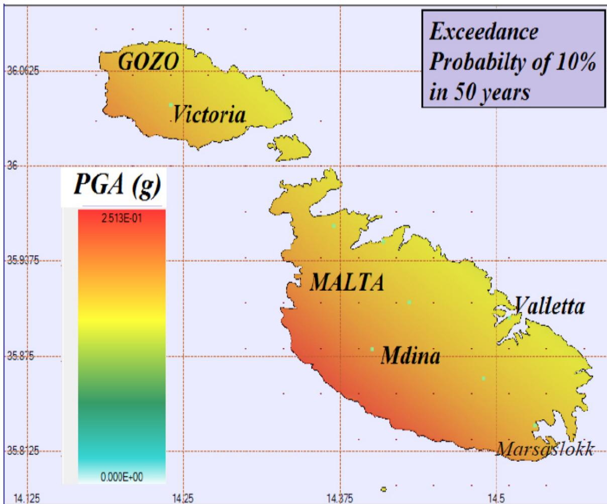
Figure 3. Preliminary seismic hazard map at the bedrock (D'Amico et al., 2013)
