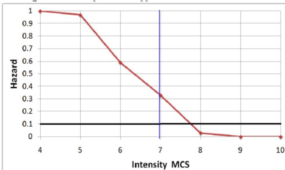
Figure 5: Hazard curve computed for the Maltese Islands using the SASHA code
