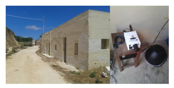
Figure 2.5: Selected station site in Ta' Cenc, at the Water Services Corporation plant. Left: The room housing the seismic station during testing. Right: The temporary set up inside the room: seismometer, digitizer, GPS receiver and an UPS for consistent power supply.
